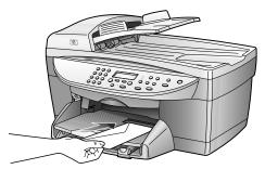
• If you are printing multiple envelopes, remove all paper from the main tray, and then slide a stack of envelopes down the right side of the tray, with the envelope flaps up and to the left (print side down), until they stop.
