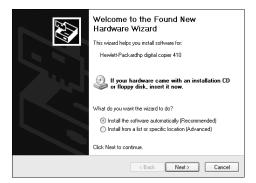
**Note:** Windows XP incorrectly identifies the HP Digital Copier Printer 410 as "Hewlett-Packardhp digital copier 410." This does not affect the success of the installation.
