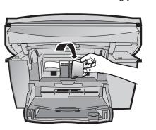
Lower the right print-cartridge latch down onto the top of the cartridge, and push down until the latch locks firmly into place.
