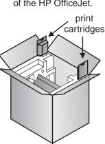
Rest the box on its side and pull out your HP OfficeJet. Remove any packaging or tape from the HP OfficeJet.
