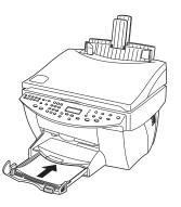
6 To prevent paper from possibly falling off the tray, pull out the output-tray extender.
