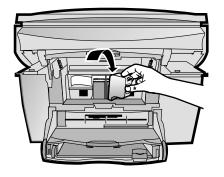
Lower the right print-cartridge latch down onto the top of the cartridge, and push down until the latch locks firmly
