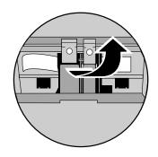
Remove the black print cartridge (thinner one) from its packaging and, being careful to touch only the black plastic, gently remove both the green pull tab and the blue tape
