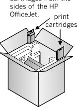
Rest the box on its side and pull out vour HP OfficeJet. Remove any packaging or tape from the HP
