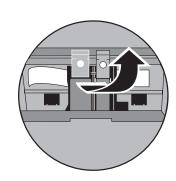
Remove the black print cartridge (thinner one) from its packaging and, being careful to touch only the black plastic, gently remove both the green pull tab and the blue tape covering the nozzles.
