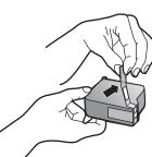
Push the color print cartridge firmly down into the slot on the left. Lower the left print-cartridge latch down onto the top of the cartridge, and push down until the latch locks firmly into place.
