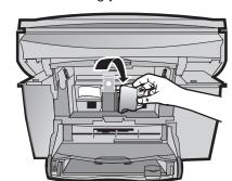
Lower the right print-cartridge latch down onto the top of the cartridge, and push down until the latch locks firmly into place.
