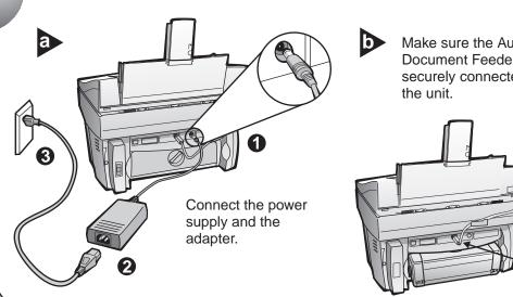
Make sure the Automatic Document Feeder cord is securely connected to
