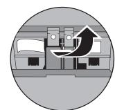
Remove the black print cartridge (thinner one) from its packaging and, being careful to touch only the black plastic, gently remove both the green pull tab and the blue tape covering the nozzles.
