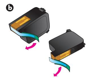
Pull the green tab to remove the blue tape from the print cartridges. Do not touch the gold-colored contacts or retape the cartridges.
