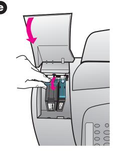
Lower the print-cartridge latches onto the top of the cartridges, and push down firmly until the cartridges lock into place. Close the print cartridge door.
