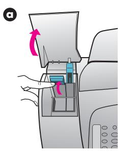
Lift the print cartridge door up until it catches. Wait for the print carriage to move into view. Lift the latches.
