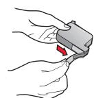
Push the black print cartridge firmly down into the slot on the right. As you insert the cartridge, make sure the label is facing you.
