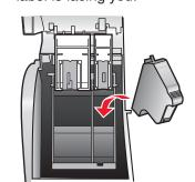
Lower the right print-cartridge latch down onto the top of the cartridge, and push down firmly until the latch locks into place.
