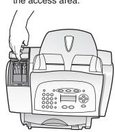
Wait at least 10 seconds for the print carriage to stop moving. Raise both latches on the print carriage.
