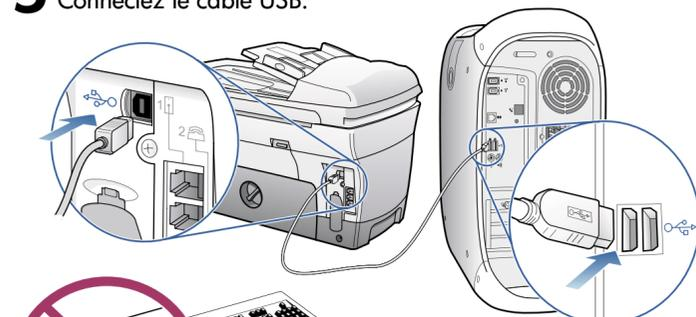
Do not connect your HP OfficeJet to a USB port on a keyboard or a non-powered USB hub. See the reference guide for more details.
