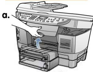
**2** Release the gray print carriage latch, and then lift the print carriage to access the printhead carriage.
