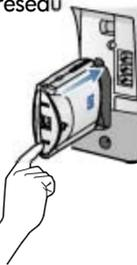
Press the button on the network adapter. A page prints with your network configuration. Locate the IP address. If the IP address is 192.0.0.192 or 0.0.0.0, then see Networking Tips. Save this sheet for step 15.
