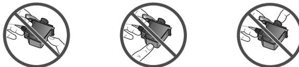
Do not touch the copper contacts, the ink nozzles, or the printhead tower.
