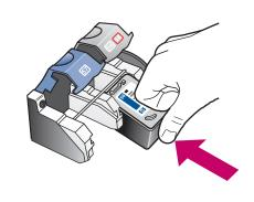
Hold the black print cartridge with the HP label on top. Slide the cartridge underneath the metal bar into the right (gray latch) side of the print carriage.
