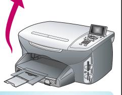
Press **OK** on the front panel to begin alignment. After a page prints, alignment is complete. Discard or recycle this page.
