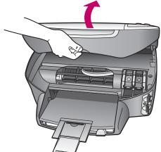
a Lift the print carriage door up until it catches. Wait for the print carriage to move to the right. Lift the blue and gray
