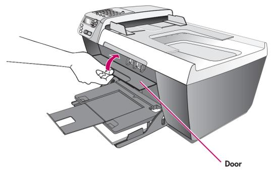
Lift the print-carriage access door. The print carriage slides to the middle.
