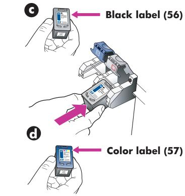
Hold the black print cartridge with the label on top as shown. Slide the cartridge into the right (gray latch) side of the print carriage.
