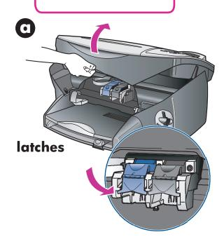
Lift the print carriage door up until it catches. Wait for the print carriage to move to the center. Lift the blue and gray latches.
