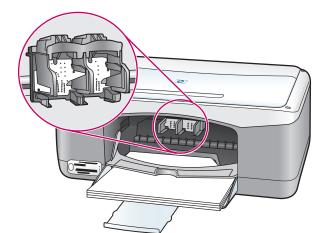
Insert and align the print cartridges
