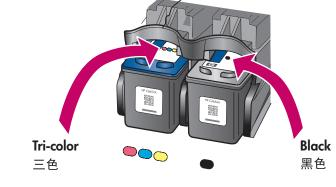
Hold the color print cartridge with the large HP label and the raised markings on top. Slide the cartridge at a slight angle into the left side of the print carriage.
