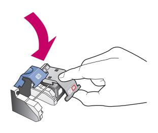
d Press down on the gray latch until it locks into place. Insert
