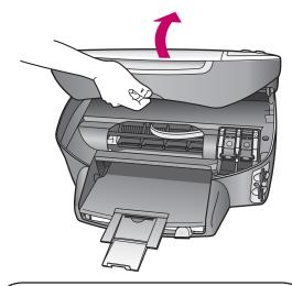
Lift the print carriage door up until it catches. Lift the blue and gray latches.
