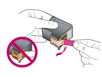
**b** Remove the bright pink tape from both the print cartridges. Do not touch the gold-colored contacts or retape the cartridges.
