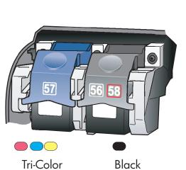
Make sure both latches are locked into position. Close the door.
