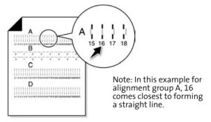
Using the same **up**, **down** and **start/yes** buttons used in step 4, change the value for the letter displayed on the printer LCD, and then press **start/yes** to select it. The next alignment letter will be shown until you have set all the alignment values for the page.
