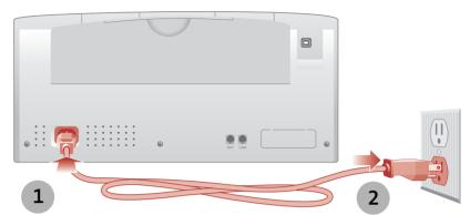
You should plug the power cord, which has a three-wire electrical grounding type plug, into a grounded electrical outlet.
