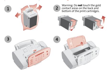
Note: The cartridge carrier moves to the loading position when you open the cover.
