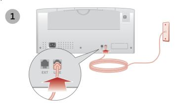
Optionally, you can attach a telephone. This lets you use the fax line as a normal telephone line.
