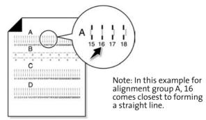
Using the number keypad, enter the value for the letter displayed on the printer LCD. The next alignment letter will be shown until you have set all the alignment values for the page.
