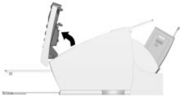
Opening the control panel
