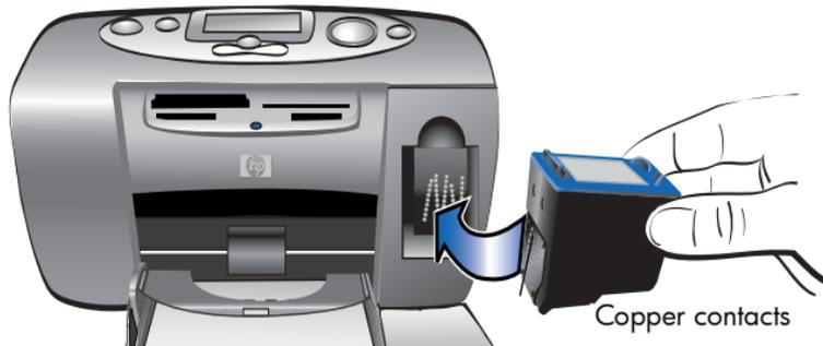
4. Push the print cartridge into the print cartridge cradle until you feel it snap into place.
