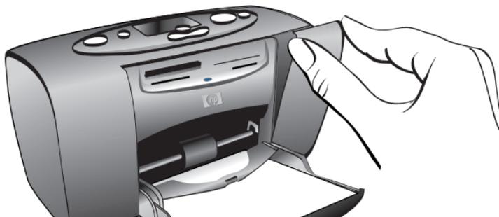
3. Place the print cartridge in the print cartridge cradle with the copper contacts facing toward the inside of the printer and the ink nozzles facing down.
