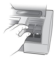
5 If you are replacing a print cartridge, slide out the old print cartridge and recycle or discard it.
