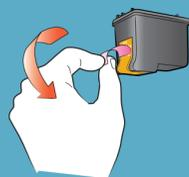
⊘ Do not touch or remove the ink nozzles or the copper contacts!
