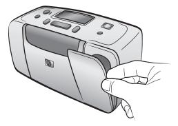
Place the print cartridge in the print cartridge cradle with the copper contacts facing toward the inside of the printer and the ink nozzles facing down.
