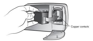
6 Push the print cartridge into the print cartridge cradle until you feel it snap into place.
