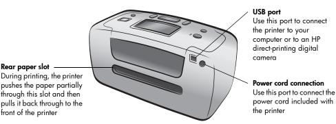
Note: Place the printer on a flat, stable surface with the back of the printer at least 10 inches (250 mm) away from any obstruction to allow space for the paper to move through the printer during printing. Make sure the power cord and USB cable do not block the rear paper path.
