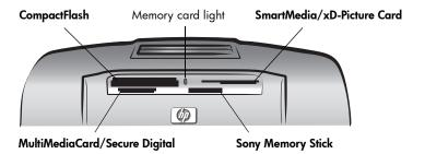
**Note:** If you are using a Sony Memory Stick Duo memory card, attach the adapter that came with the memory card before you insert it into the printer's memory card slot.
