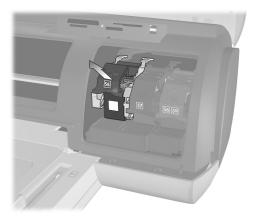
5 If you are replacing a print cartridge, slide the old print cartridge out and store, recycle, or discard it.
