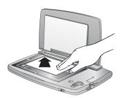
Macintosh scan: When the light stops blinking, the Photos Remaining indicator on the scanner will decrease. Follow the instructions in the **HP Image Unload** dialog to unload the images. The HP Image Unload software saves the image to the hard disk, then asks if you want to browse the image. If you choose to browse, the image will appear in the HP Photo and Imaging Gallery.
