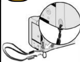
1. Thread the short loop of the wrist strap through the wrist strap attachment. You might need to use a paper clip to thread the end of the loop through.
