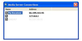
If you wish to be prompted before allowing a receiver access to shared content on the server PC, uncheck the **Allow Clients By Default** box. Whenever you attach a new receiver, a message box will appear on the PC asking whether you wish to allow access.
