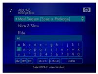
To use the keyboard, highlight a character with the arrow buttons and press **select**. Highlight and select **Done** when you are finished entering text.
