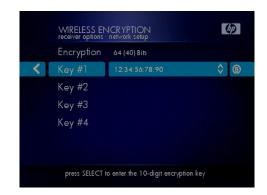
Some network devices allow the use of a text passphrase for the WEP key. After you enter the passphrase on that device, view the encryption keys that were generated. Write down the keys and enter them into the **Key** fields on the media receiver.
