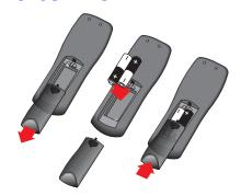
Place the included batteries in the remote control.
