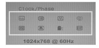
**3** If 'Clock' is selected, you may use the '+' or '-' buttons to adjust the setting of clock. The fullness of the graphic bar as well as the numerical value at the right corner is changed accordingly.
