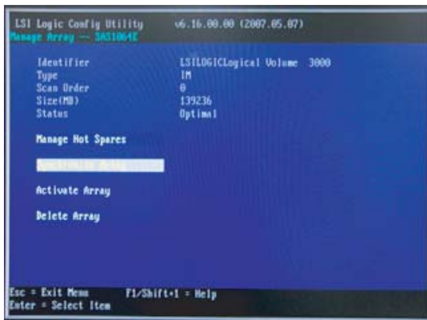
Figure 6-7 LSI Logic MPT Setup Utility – Manage array
