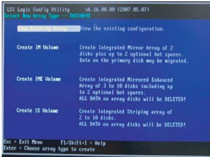
Figure 6-4 Logic MPT Setup Utility – RAID properties
