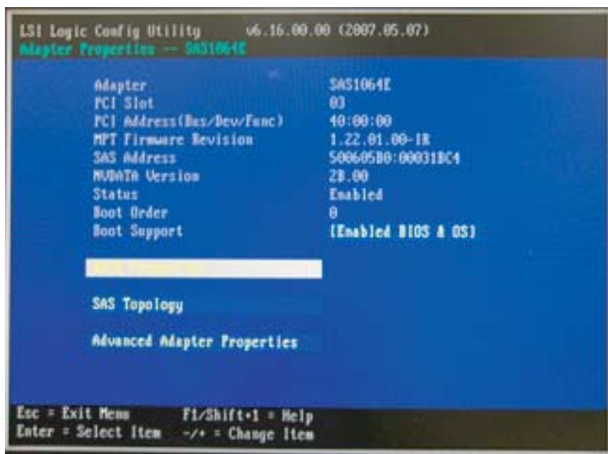
Figure 6-3 LSI Logic MPT Setup Utility – Adapter properties
