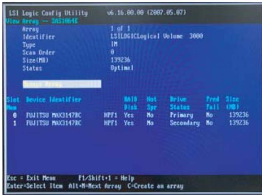
Figure 6-6 LSI Logic MPT Setup Utility – View array
