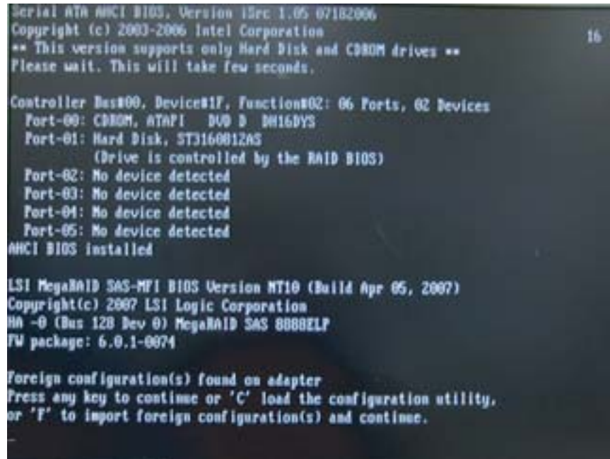
Figure 6-13 Foreign configuration on LSI adapter
