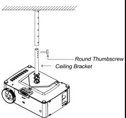
4 Make necessary roll and yaw adjustments to the projector.
