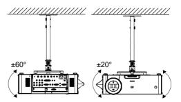
Open the on-screen menu and select Setup > Projector Position. Select the appropriate ceiling option.
