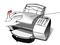
Open the cover. The empty print cartridge holder moves into view.
