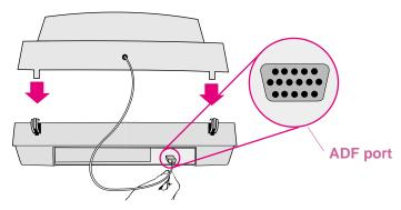
**c** Attach the input tray to the ADF. Insert the tabs on the input tray into the slots on the ADF. Gently push the input tray until you hear a click.
