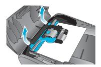
4 While lifting the green lever, rotate the pick mechanism until it stays open.
