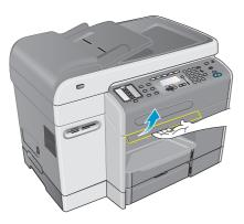
4 Remove the keyboard tray lock from the underside of the print-carriage access door.
