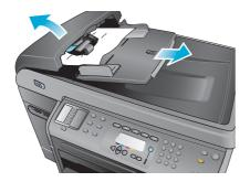
3 Remove the jam cleanout part. Using both hands, lift up on the two handles until the part unsnaps. Rotate and lift out the cleanout and set it aside.
