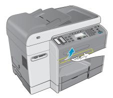
**a** When you lift the print-carriage access door, the carriage should return to the right side of the all-in-one. If the carriage does not return to the right side, turn off the all-in-one.
