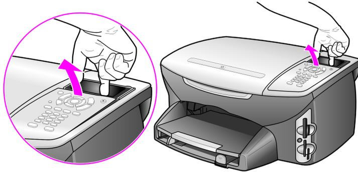
**Tip:** You can also use a thin, flat object, such as a credit card, to lift the front panel cover. Gently slide the credit card at a slight angle, about 45 degrees, between the color graphics display and the front panel cover. Apply slight downward pressure to lift the front panel cover.
