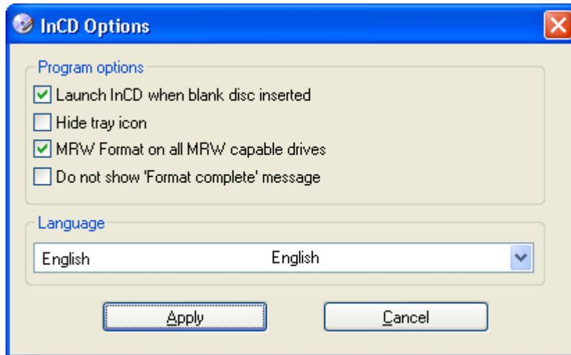
Unlike CD-RW and DVD-RW discs, MRW discs can be written on after only about one minute of formatting. This does not mean that the MRW is fully formatted after two minutes, but simply that it is formatted sufficiently for you to be able to copy data on it. The remainder of the formatting will continue in the background.
