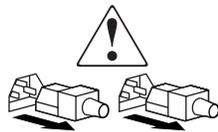
**WARNING:** To reduce the risk of injury from electric shock, remove all power cords to completely disconnect power from the system.
