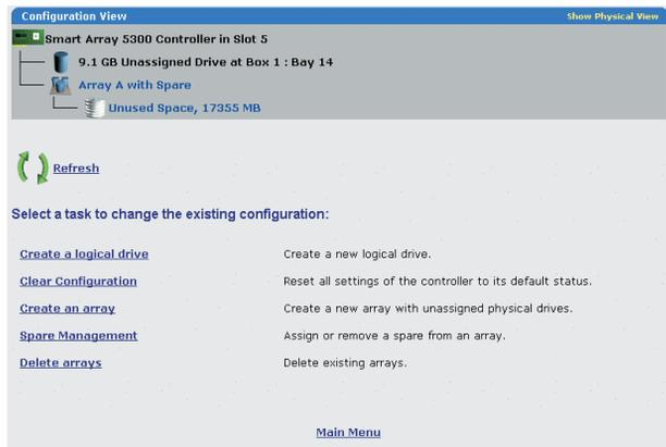
**Figure 2-5: Configured array screen (no logical drives)**
