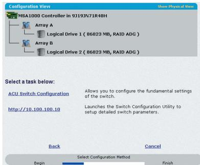
**Figure 3-7: Launching the Switch Configuration Utility**
