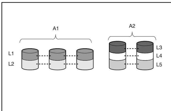
**Figure A-4: Two arrays (A1, A2) containing five logical drives spread across five physical drives**
