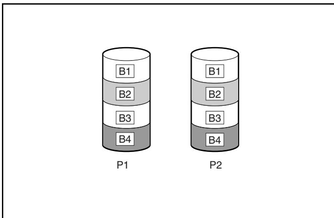
**Figure A-5: Drive mirroring of P1 to P2**
