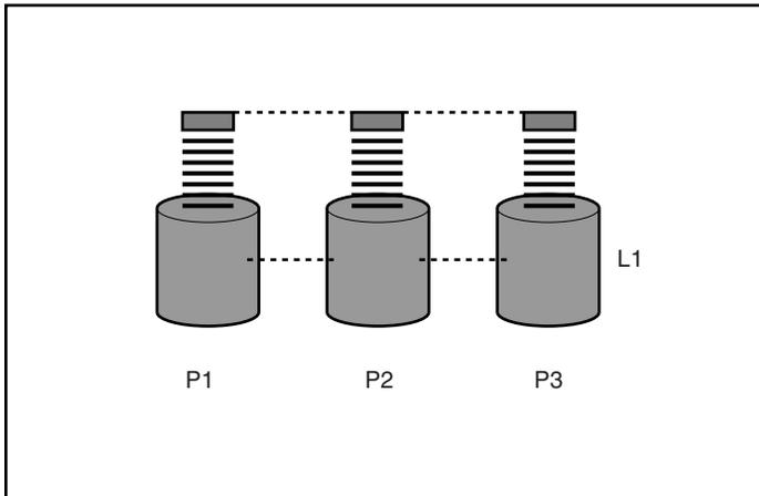
**Figure A-2: Physical drives configured into a logical drive (L1)**
