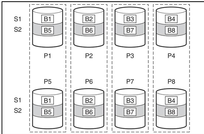
**Figure A-6: Mirroring with more than two physical drives in the array**
