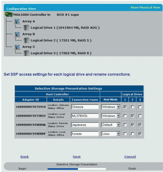
Figure 3-3: Typical SSP screen for the MSA1000
