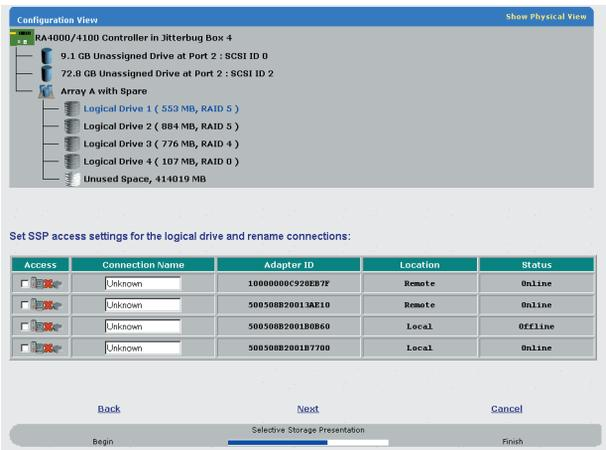
Figure 3-2: Typical SSP screen for the RA4x00
