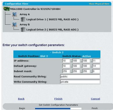
**Figure 3-6: Setting switch parameters**
