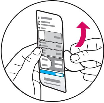
**a** Remove the adhesive backing from the control-panel overlay.
