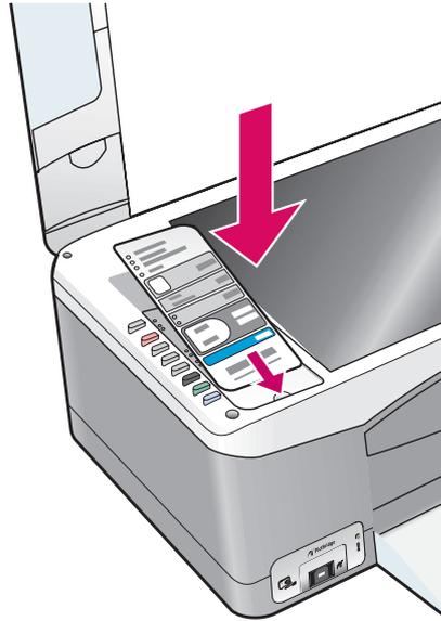
**b** Raise the lid. Place the control-panel overlay into the recess. Make sure it sticks in place.
