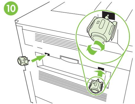
10 Position the metal alignment brackets and magnets in front of the printer's cap holes and attach the brackets by inserting and screwing the magnets.
