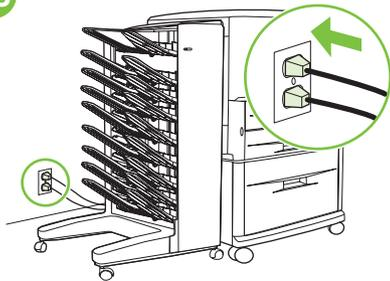
Reconnect the power cord for the printer to the ac power outlet. Reconnect the power cord for tray 4 to the ac power outlet.
