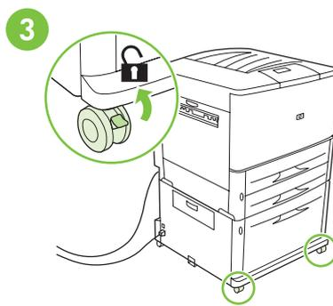
Unlock the printer front wheels.
