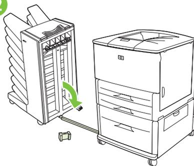
Lower the connecting rod to a horizontal position.
