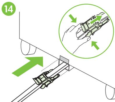
Slide the blue plastic bracket into the metal slot until it locks into place.
