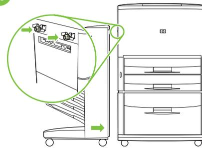
Push the 8-bin mailbox toward the printer. The 8-bin mailbox should slide in to touch the two magnets on the printer and lock the 8-bin mailbox into place.
