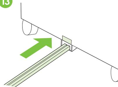
Put the end of the connecting rod into the U-shaped metal slot on tray 4 and align the rod with the grey alignment label.
