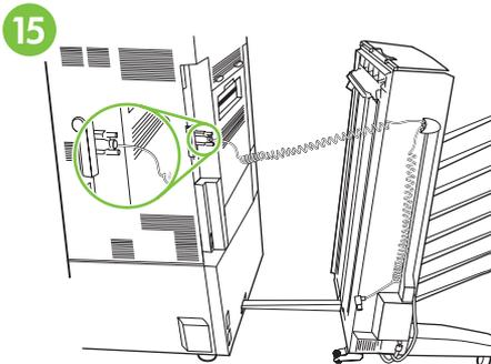
Securely connect the communication cable to the printer at the connector labeled "Accessory".
