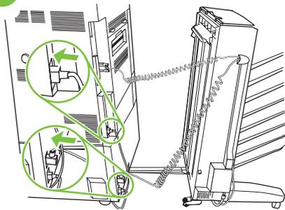
Connect the power cord for the printer to the printer. Connect the power cord for tray 4 to tray 4.
