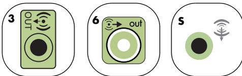
**3** Connect the rear speaker cable to the black connector that matches the back of your PC.
