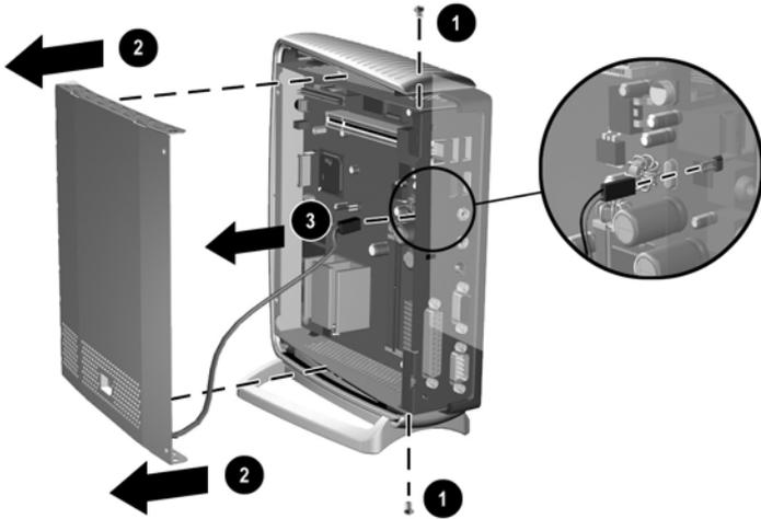
*Removing the Chassis Cover and Disconnecting the Speaker*
