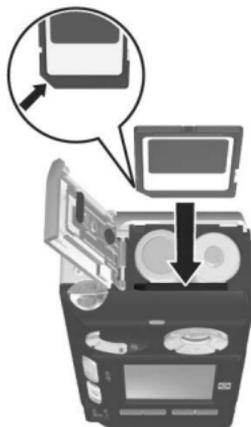
To remove the memory card from the camera, first turn the camera off. Then open the Battery/Memory card door, press down on the top edge of the memory card, and it will spring outward from the slot.
