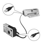
Connect the square end of that USB cable to the HP Photosmart printer.
