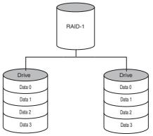
The cost of this redundancy is inefficient use of capacity, because all data is written to both drives, only half of the total capacity is available.
