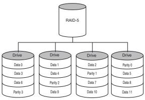
Using parity minimizes the capacity cost of redundancy. Since only one drive is used to store parity, the worst case of a three-drive RAID-5 only loses one third of the total capacity, for arrays with more drives the lost capacity is smaller.
