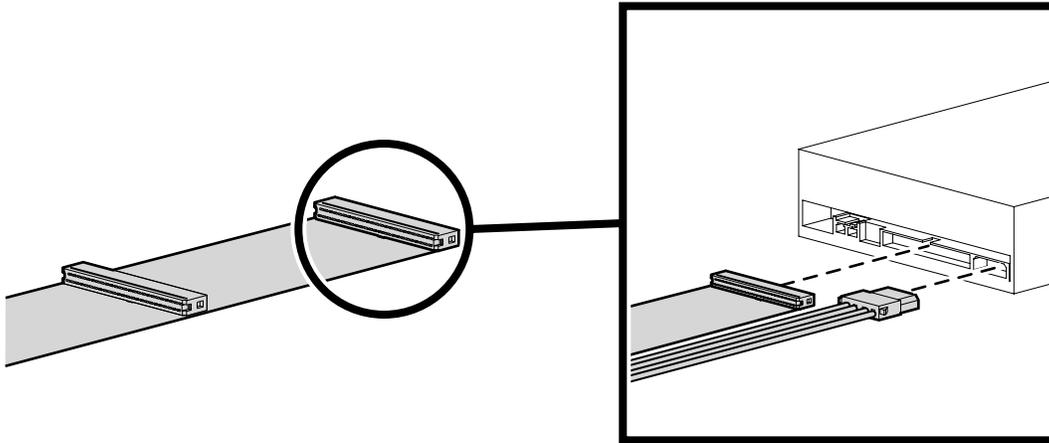
**Note:** Use the connector at the end of the cable to connect to the drive. Some cable may have more than one connector; however, only one connector is needed to connect to the drive.
