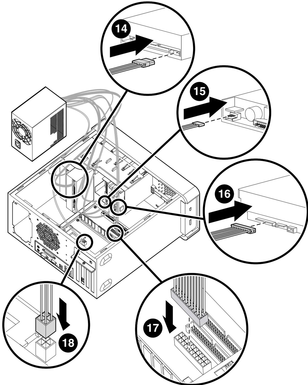
**All connectors are keyed for their intended location and should not require excessive force to plug in.**
