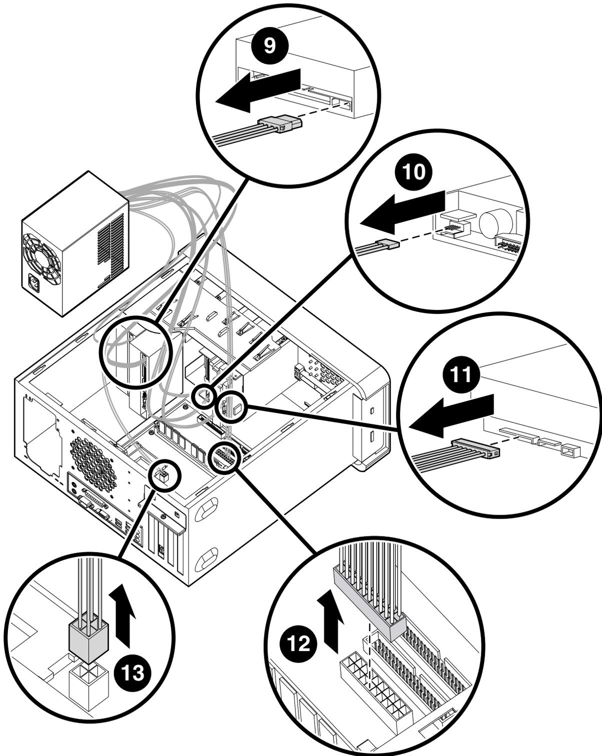
Identify where the power supply cables are connected before you unplug them.
